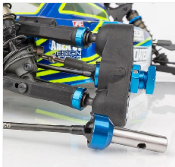
#81590 FT CVA Axle Sleeves installed
