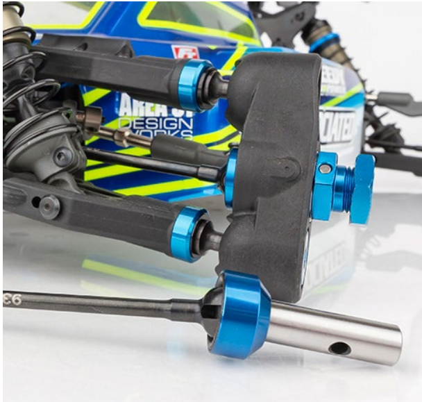
#81590 FT CVA Axle Sleeves installed
