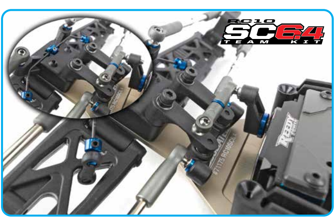
New adjustable height steering system. SC6.2 is not adjustable
