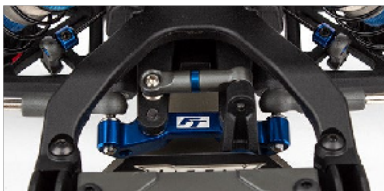
#91984 Steering Rack mounted in the RC10B6.4
