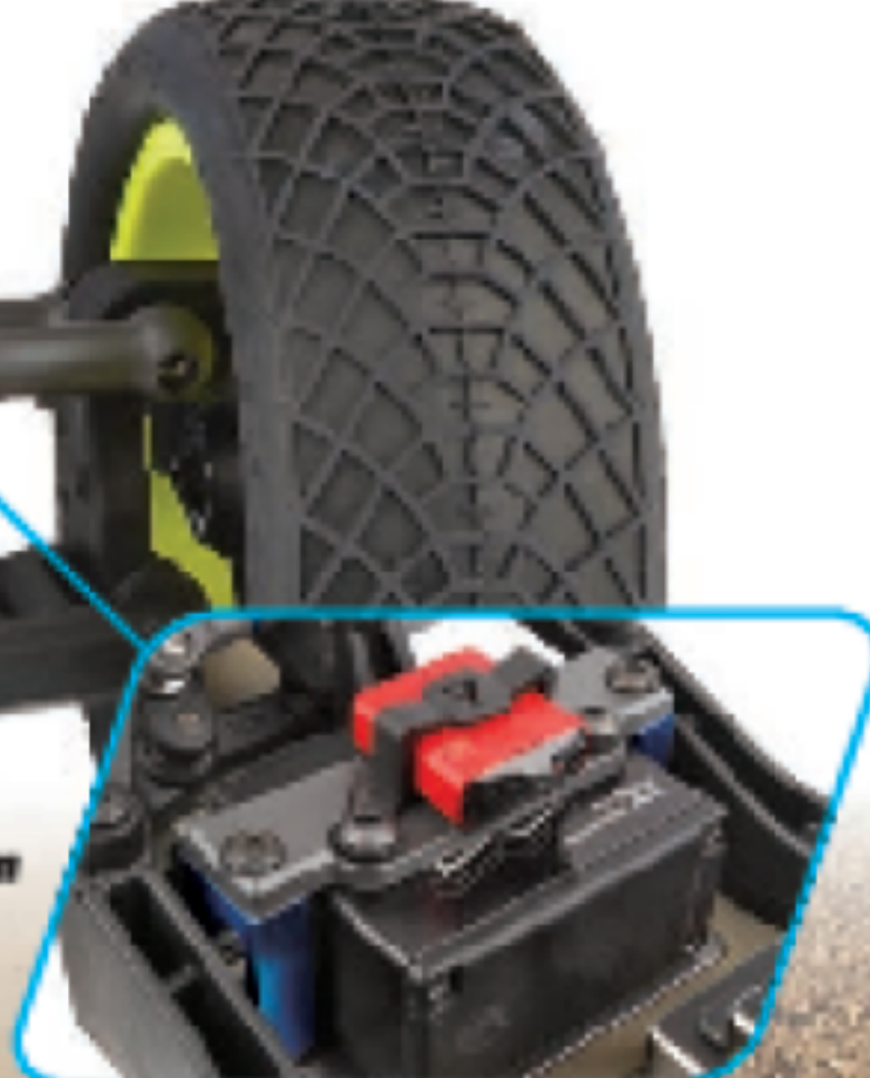
NEW direct-to-chassis aluminum servo mounting system
