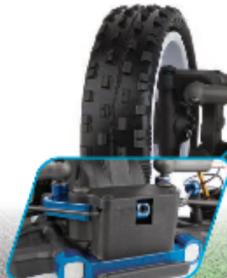
Front and rear anti-roll bars for less body-roll and more traction on high grip surfaces
