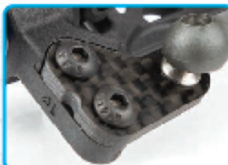
Carbon fiber +1 steering plates
