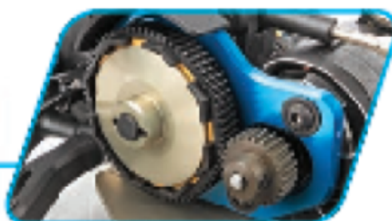
Octalock spur gear and 19mm LCF pads
