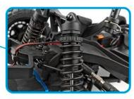
Threaded, fluid-filled, coil-over shock absorbers
