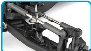
Rugged steel turnbuckles for adjustable camber and front toe-in
