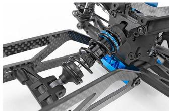
With a rigid wheelie bar, it is possible for the car's rear tires to lose traction when the wheelie bar wheels abruptly hit the ground. With this conversion, you'll dampen this impact, allowing for greater traction and control at launch without sacrificing the main function of the wheelie bar.
