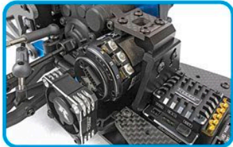
Mid-motor design creates improved traction and control in the vehicle's weight distribution
