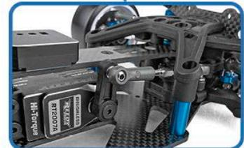
Carbon fiber upper deck provides two servo mounting options for adjustable weight balance.
