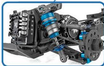
Our race-proven threaded aluminum oil-filled shocks work with the chassis design to provide exceptional tuning options
