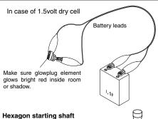
This shaft mounted on an electric starting motor is driven into the shaft cup to turn the engine.
