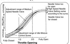
NOTE: With this carburetor, neither the Idle Mixture Control Screw adjustment, nor the Medium Speed Needle Valve adjustment will have any effect on mixture strength when the throttle is fully (or almost fully) open.
