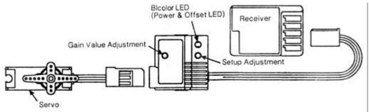
Disconnect the servo to be compensated from the receiver and plug the connector from the gyro there, then insert the servo connector to the gyro port. Be sure to observe the proper polarity on the connector and the gyro port (socket). If the wires on the components are excessively dragged each other, it is not possible to get best vibration absorption with the mounting foam tape, also it may cause possible disconnection during use.
