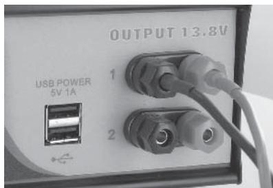
4mm bullet connectors plug directly into most power supplies.
