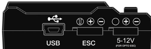
Connect the PROcontrol controller to the PROcontrol programmer. The respective port is labeled ESC. Use the right connection cable and ensure correct polarity. ROXXY PROcontrol controllers come with two connection cables. Use the three-wire cable for connection to the programmer.
