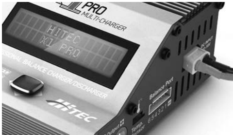
XT60 Connector plugged directly to charger.
