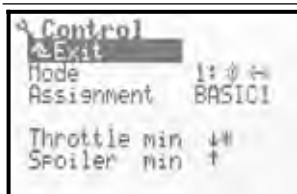
Fig. 1: SETUP/Control menu for fixed-wing models
