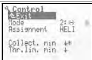
Fig. 2: SETUP/Control menu for model helicopters
