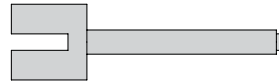
86015 Ⓞ Gear Diff Shaft 5x35mm Sprint Kegeldiffachse Axe de pignon differential ギヤデフシャフト
