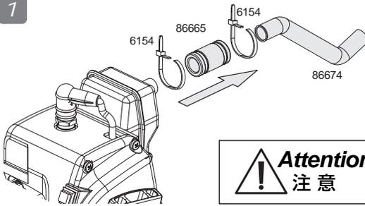
Remove the #86674 Exhaust Pipe before tuning the engine. Be sure to remove it when the exhaust has cooled down. With the exhaust pipe removed, you can feel the response of the engine better, this will make it easier to tune the carburetor. By removing the exhaust pipe, you can get maximum power from the engine. If the engine is too loud after tuning, re-install the exhaust pipe.
