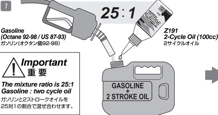
You must only use a mixture of gasoline and two stroke oil as fuel for this engine.
