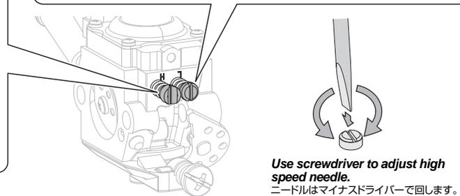
Use screwdriver to adjust high speed needle.
