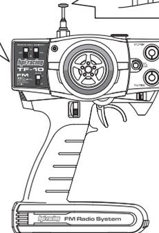
**! If you switch off the transmitter first before the R/C car, you may lose control of the R/C car.**
