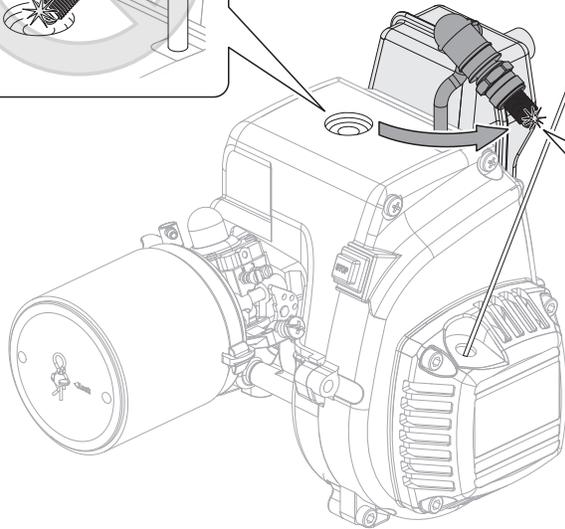
Check if spark plug is firing.
