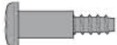
Z282 Step Screw M3x14mm Stufenschraube M3x14mm Vis M3x14mm ステップスクリュー-M3x14mm
