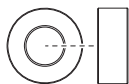
102823 a Plastic Bushing 5x10x4mm Plastiklager 5x10x4mm Bague plastique 5x10x4mm プラッシュ 5x10x4mm
