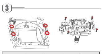
3. Loosen the assembly screws shown in fig.4 and remove the plate. Be careful to ensure no damage to cables.
