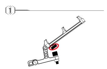
1. To adjust the bracket, loosen locking screw by turning it anti-clockwise.
