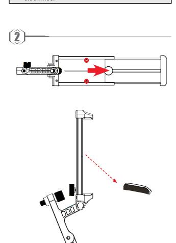
2. Move the slide to the highest position and remove the screws marked in red.
