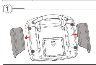
1. Use tweezers to remove the left and right hand grips. Then use a screwdriver to remove the 4 screws marked in red.
