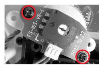
2. Remove the PCB screws marked in red.
