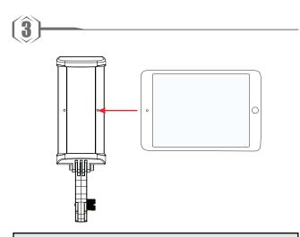
3. Move the your device into the centre of the bracket. Be careful not to let the device fall.
