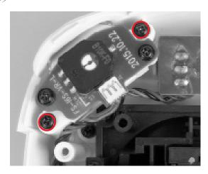
1. Take the transmitter apart, then use a screwdriver to remove the screws marked in
