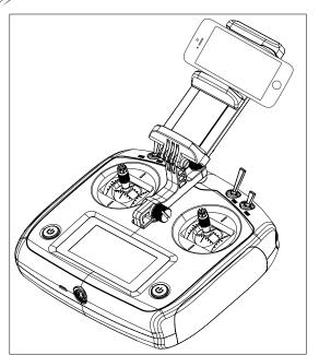
$5. \ \ \, \text{Tighten the lock screw on the back of the bracket}.$
