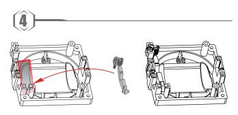
4. Place the spring hook assembly into position and hook the spring onto the hook located inside the transmitter.
