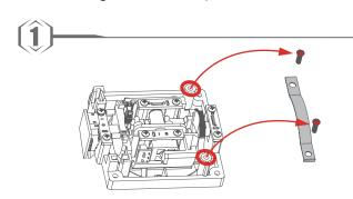
3. Take the transmitter apart, then remove the screws marked in blue and remove the bracket.
