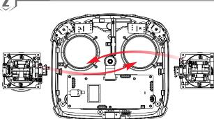
2. Swap the gimbals and rotate them 180 degrees, then line them up with the screw holes and replace the screws. (There is no need to disconnect the cables.)
