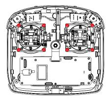
1. Take the transmitter apart, using a Philips screwdriver, remove the 8 screws marked in red.
