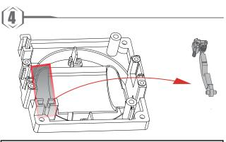
4. Remove the bottom of the seat assembly of the spring hook assembly.
