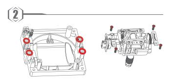
2. Loosen the screws shown in fig.4 and remove the plates.
