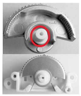
4. Please the spring as marked in red with the 2 ends pinched between the plastic at the bottom.
