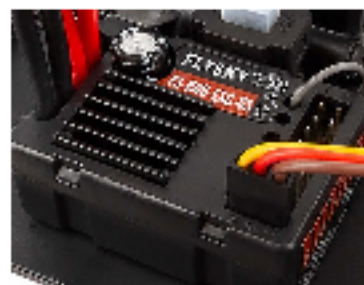
2-in-1 ESC/receiver unit
