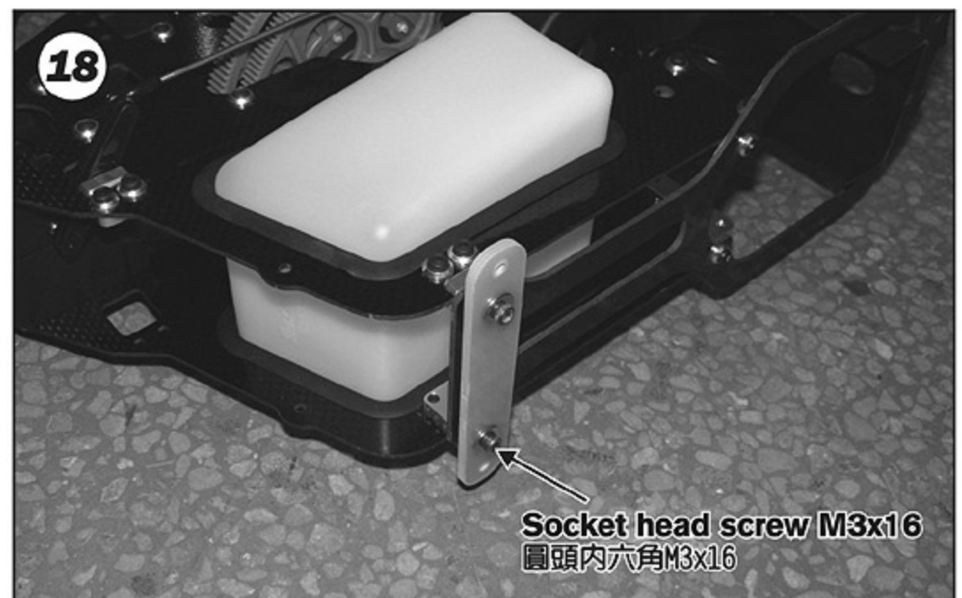
18 Fasten the spacers and fixing plate to the bottom plate with socket head screws M3x16 and washer \Phi 3.4 \times \Phi 9.9 \times \Phi 0.9 mm. 以圓頭內六角螺絲M3x16與華司 \Phi 3.4 \times \Phi 9.9 \times \Phi 0.9 mm將墊片和固定片鎖附於底板。
