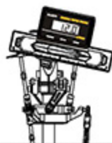
Stick Position at High/Throttle 100%/Pitch+12° 搖桿高速/油門100%/Pitch+12°
