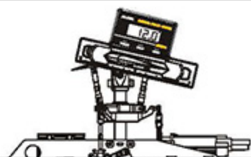
Stick position at high/Throttle 100%/Pitch+12° 搖桿高速/油門100%/Pitch+12°
