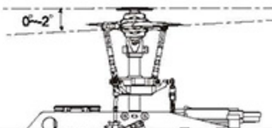
Stick position at low/Throttle 0%/Pitch0~-2° 搖桿低速/油門0%/Pitch0~-2°
