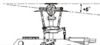
Stick position at Hovering/Throttle 70%/Pitch+5° 搖桿停懸/油門70%/Pitch+5°
