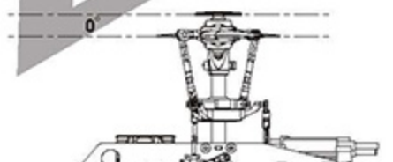
Stick position at middle/Throttle 90%/Pitch 0° 搖桿中速/油門90%/Pitch 0°
