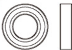
Bearing 軸承 (φ 12x φ 24x6mm) x 3
