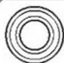
Bearing 軸承 (φ10xφ19.5mm) x2
