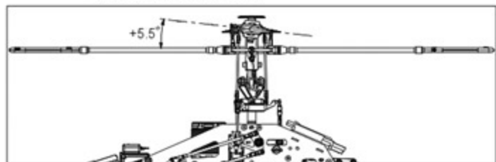
Stick position at Hovering/Throttle 70%/ Pitch+5.5° 搖桿停懸/油門70%/Pitch+5.5°
