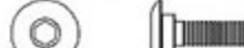
Socket button head collar screw 半圓頭內六角軸套螺絲 (M3x8mm) x 4
