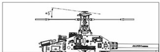
Stick position at Hovering/Throttle 60%~65%/Pitch +5° 搖桿停懸/油門50%-65%/Pitch+5°
