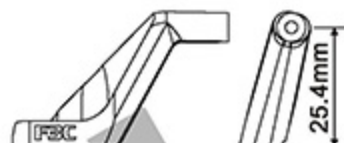
[H76H002XXW] 760X F3C Main Rotor Holder Arm 760X F3C主旋翼夾座臂
