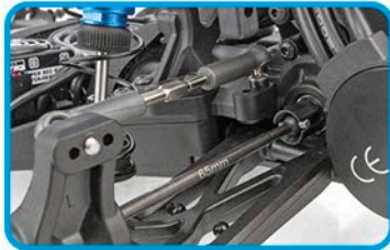
65mm rear CVA drive shafts for reliability
