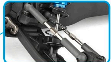
Rugged steel turnbuckles for adjustable camber and front toe-in
