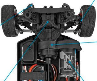
A sealed center driveline keeps dirt and debris out--along with bits of tire rubber--for smooth and reliable power delivery
